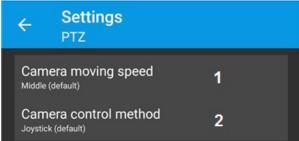
2. Select PTZ camera control mode (2, see Controlling PTZ cameras from the Android Mobile Client): step keys or a virtual joystick.
