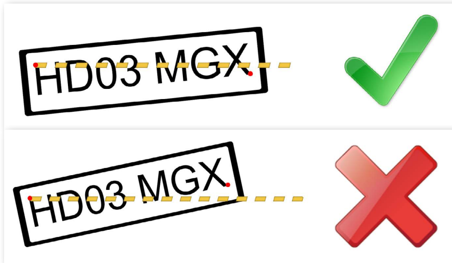
Figure 9 – Determining allowed tilt of the license plate (“rule of one line”)
