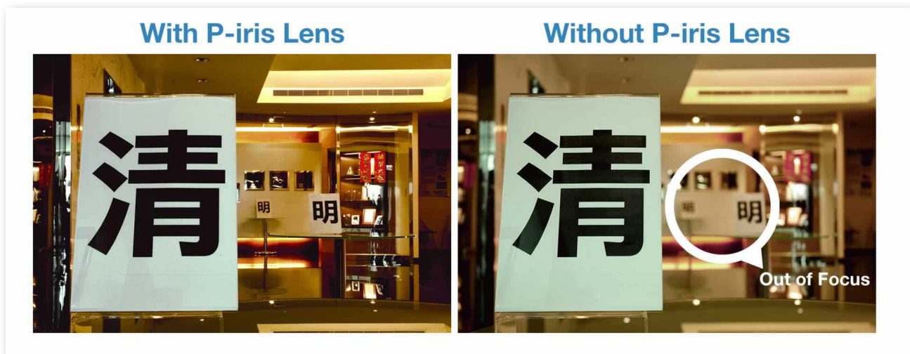
Figure 5 – Comparing sharpness of images taken with and without P-iris 3
