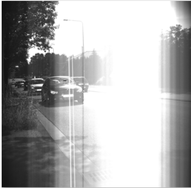
Figure 3 – Example of an image with rolling shutter
