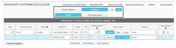
By default, the platform is calculated for a 64-bit system and 64-bit modules. When using cameras that do not support the x64 mode (outdated camera models, the full list is available in Documentation Drivers Pack) or when installing the software on a 32-bit operating system, select x32 mode.
