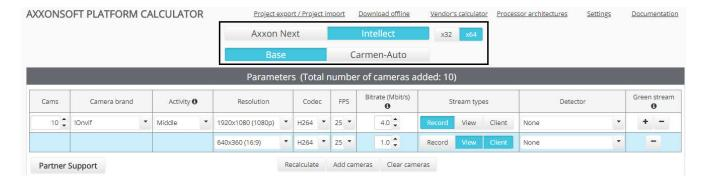
By default, the platform is calculated for a 64-bit system and 64-bit modules. When using cameras that do not support the x64 mode (outdated camera models, the full list is available in Documentation Drivers Pack) or when installing the software on a 32-bit operating system, select x32 mode.
